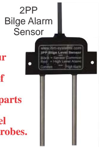
**This system can utilise either our 2PP bilge alarm sensor or float switches to measure the depth of water in the bilge. Our 2PP sensor has no moving parts to break or give trouble. Alarm operates when water level reaches the bottom of the 2PP probes.**
