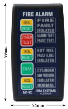
The compact sealed FA1 Fire Alarm Control Module has a dash footprint of 54 x 99 mm, is flush mount,125mm deep. Dash cut out 44x92mm
