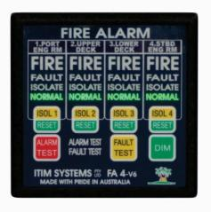
The amber **ISOLATE** indication, indicates that the Audible Alarms and Remote Alarms are isolated for that Zone. The red **ALARM TEST** indication illuminates when the **ALARM TEST** Switch is operated. The amber **FAULT TEST** indication illuminates when the **FAULT TEST** Switch is operated.
