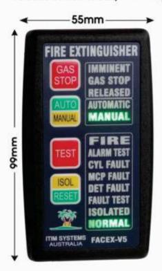
The compact sealed FACEX-V5 fire alarm and fire extinguisher control module has a dash footprint of only 55 x 99mm, a dash cutout of 44x92mm, is flush mount & 130mm deep.
