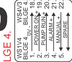
The bilge status from four bilge compartments along with remote manual pump controls connect to the two 12way terminals on the rear of the WS4-v3 bilge control module.
